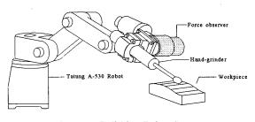
Figure 1 Polishing Robot System
